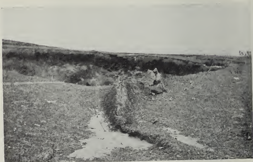
FIG. 11.—Buckling of frozen sod due to compression along the axis of a basin or sag. The movement occurred over a large excavation in a shallow mine. The sod in the foreground was lifted as much as two feet.
